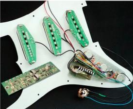
Langcaster invented the world's first real low impedance pickup being a mere 120 Ohms. This was obtained by use of a tenth of the number of turns compared to conventional pickups. This makes the inductance at least a 50th that of a conventional pickup. Self-resonance is as high as  $56 \, \text{KHz}$  - way beyond the range of human hearing. As a bonus the pickup are much more resistant to corrosion and damage and like all Langcaster pickups these are wax sealed.
